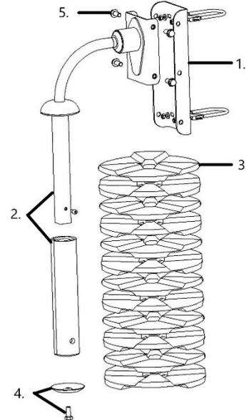
The brush device must be checked daily for observable damages to ensure a general service condition. Worn-out and damaged parts must be replaced by new genuine parts. Brush discs must be replaced if they are broken, worn-out or not cleaning efficiently.
