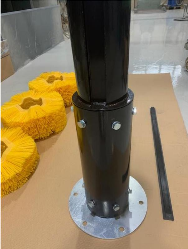
4. Add the 25 brush discs so, that the lowest disc is the pins upwards, and the next ones mirrorways. The two last discs are installed the pins downwards.
