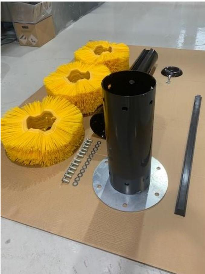
3. Attach the Upper Frame to Lower Frame with 16x30 mm Bolts and washers.
