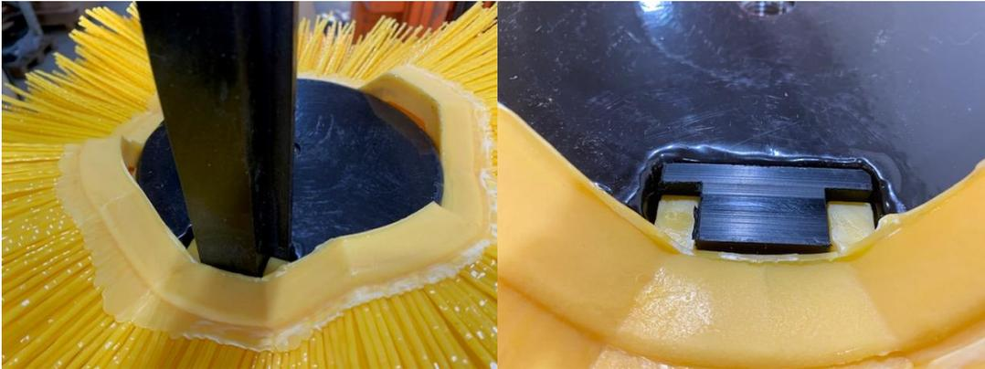
6. Install the Tensioner Lid with the DriLoc bolt and shouldered washer. Tighten all the bolts.
