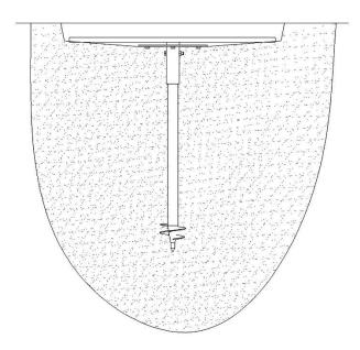
Step 5: Install the Floor Stand on the plywood plate with 16x80 mm bolts. Tighten the bolts carefully. Install the Brush into the Floor Stand and tighten the bolts carefully. Shovel some dirt on the plywood plate so that it will not be too slippery for the animals.
