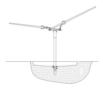
Step 3: Tighten Ground Installation Pole so, that the installation plate is attached to solid ground.
